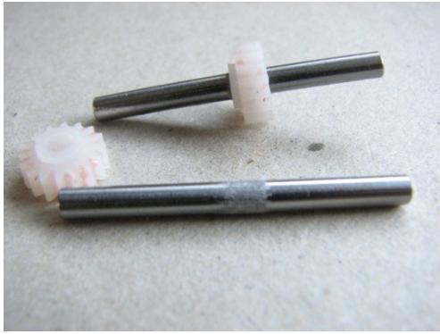
Gear on new axle – note boss faces chassis centre, plus second axle prepared for the gear.
