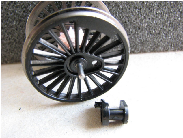
Bachmann outside cranks unplug from wheels.
