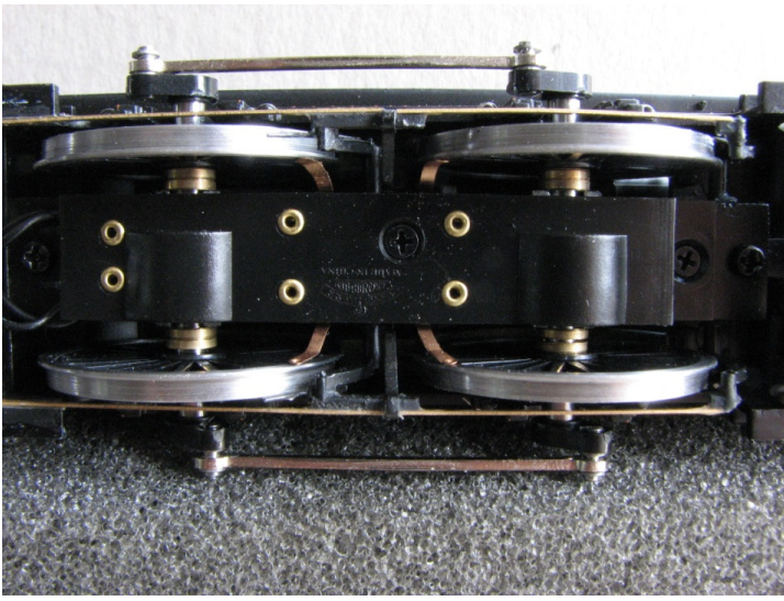
Underneath view showing new brake rods, and clearance gained.
